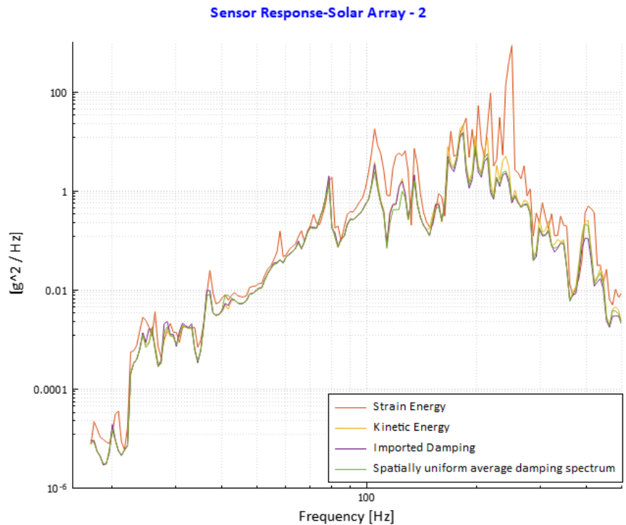
Figure 7 - Solar Array 2 location structural response comparison for the four damping distribution models
