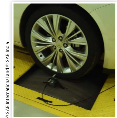
FIGURE 6 Example of transfer functions measurement test set-up for tires
