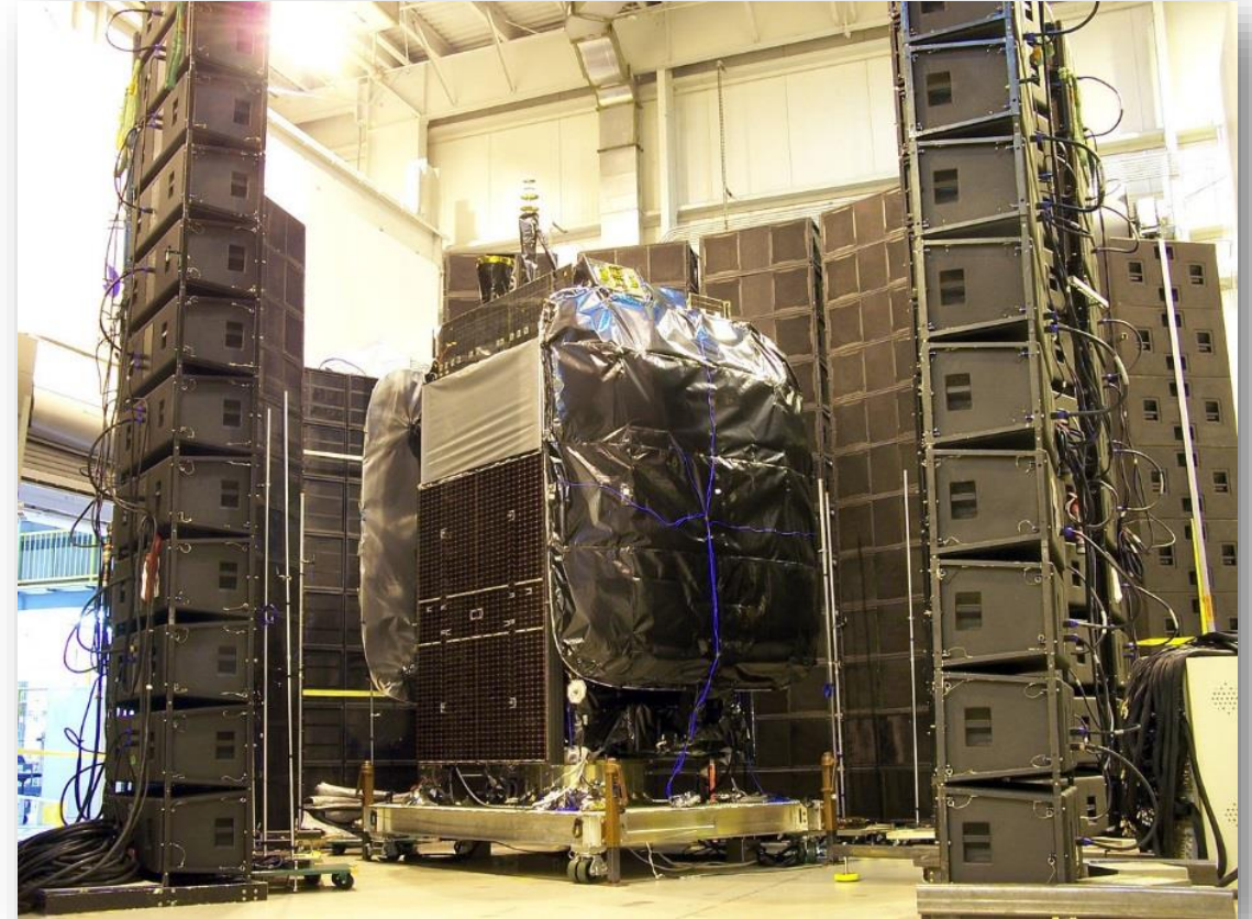
Typical Spacecraft DFAT® Test - Maryland Sound International (courtesy of Orbital Sciences Corporation) – Public Domain
