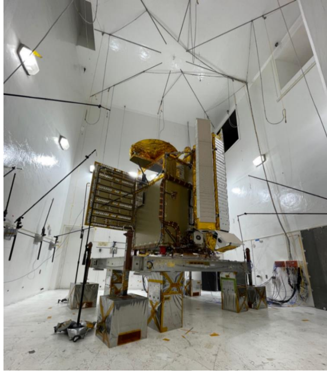
Fig. II-1 SWOT Payload Configuration in Acoustic Chamber
